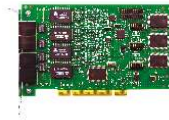
SwyxGate with up to 8 voice channels based on a Quad Basic Rate PC Card
